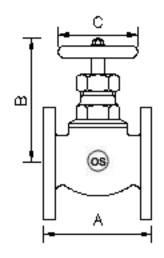
TESTING HYDROSTATIC: BODY: 24 Kg/Cm<sup>2</sup> SEAT: 16 Kg/Cm<sup>2</sup>
