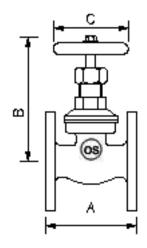
TESTING HYDROSTATIC: BODY: 24 Kg/Cm<sup>2</sup> SEAT : 16 Kg/Cm<sup>2</sup>
